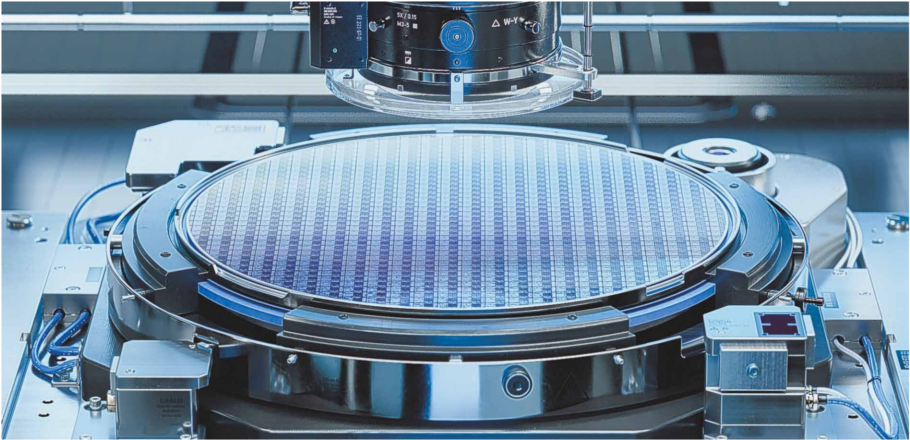
A silicon wafer—the thin, circular foundation used to manufacture computer chips—undergoes the photolithography process at a semiconductor fabrication facility.
