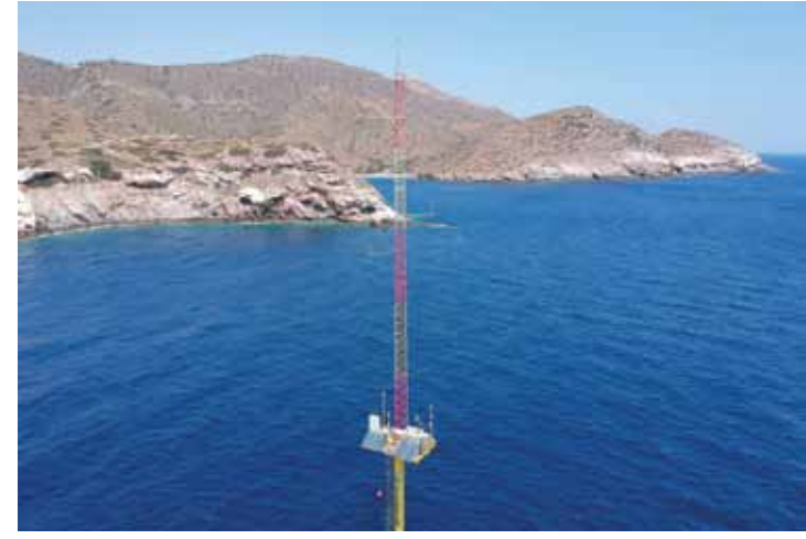
FloatMast platform in the Aegean Sea completing a 12 month wind data measurements campaign initiating Offshore Wind in Greece.
